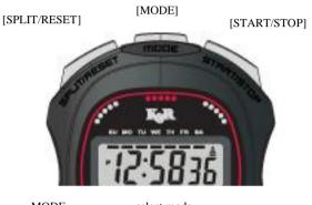
MODE START/STOP SPLIT/RESET select mode start/stop time measuring lap splitting
